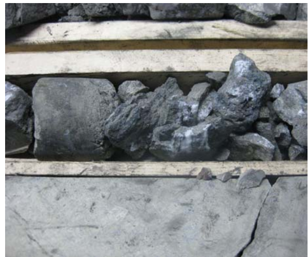
Figure 2: Hole 121 Top Oxidized Section
